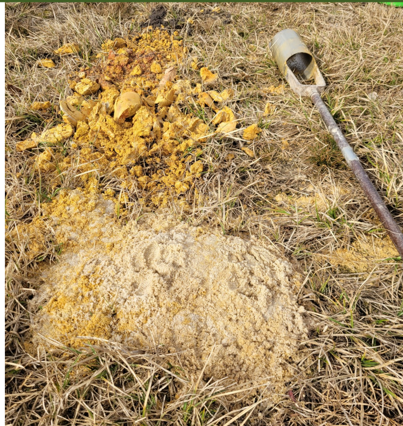
Soil sample collection of the retrofitted Lakewood Blue Claw's FirstEnergy Park basin, to monitor soil health.
