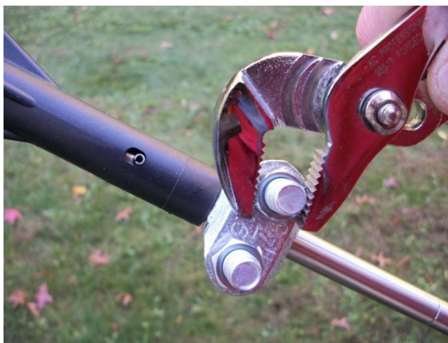
Figure 5: Removal of the locking ring. (Photo Credit: Steve Yergeau)
