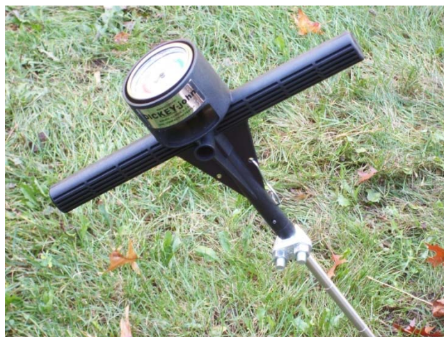
Figure 2: Soil compaction tester with locking ring in place. (Photo Credit: Steve Yergeau)
