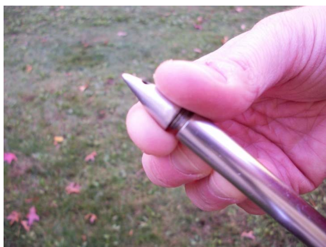
Figure 3: Installation of the soil compaction tester tip. (Photo Credit: Steve Yergeau)
