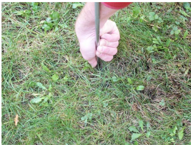
Figure 8: Grip the instrument rod and remove it from the soil. (Photo Credit: Steve Yergeau)
