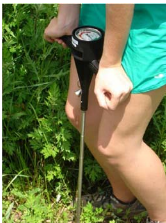
Figure 6: Proper technique for starting the soil compaction assessment. (Photo Credit: Steve Yergeau)
