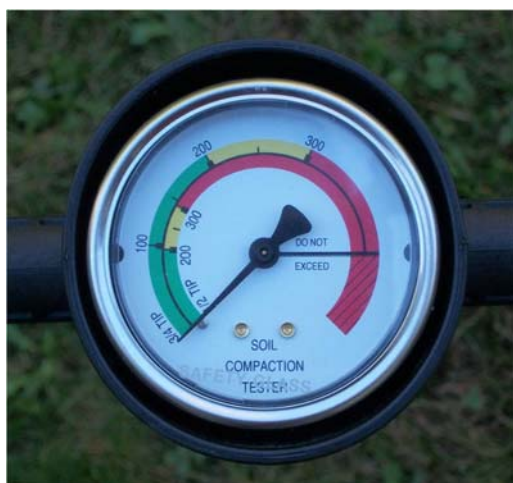
Figure 7: DICKEY-john® soil compaction tester pressure gauge showing the inner and outer scales for the ½ inch and ¾ inch instrument tips, respectively. (Photo Credit: Steve Yergeau)
