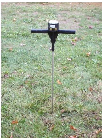
Figure 1: Static cone penetrometer, a.k.a. soil compaction tester. (Photo Credit: Steve Yergeau)
