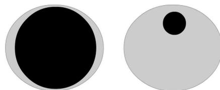
Figure 3. Two lid designs for trash can rain barrel. On the left, the majority of the lid is cut off to expose a greater screened area while the right lid only has a small opening for the downspout.
