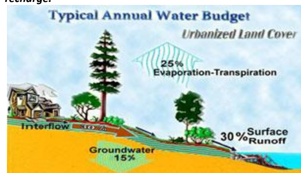
Developed Condition: notice 30% runoff and 15% groundwater recharge.
